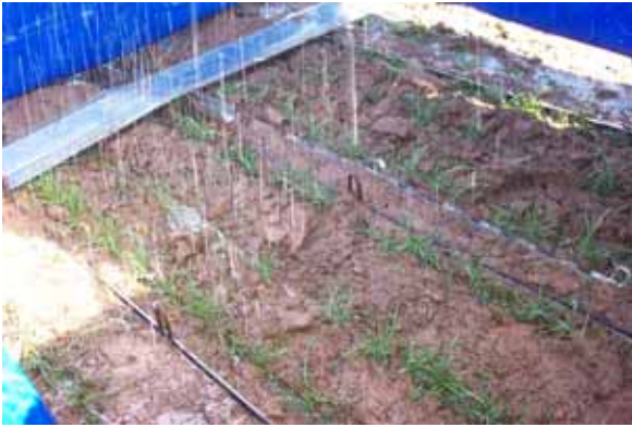
Above: Inside the rainfall simulator whilst in operation at the long-term agro-ecological trial site at the Rutherglen Research Institute.
