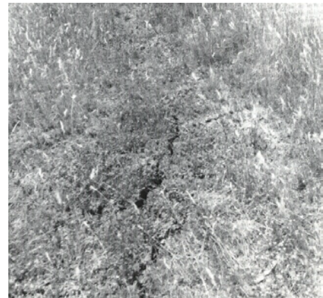
Cultivation and constructional practices are often hampered by the high shrink-swell characteristics of these clay soils.
